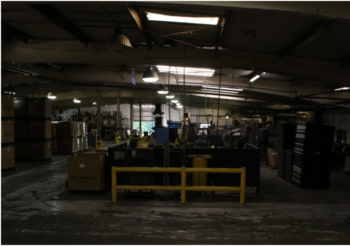
The low lighting conditions at Plastic Products of the South caused safety concerns for employees. IES recommends having at least 50 foot-candles to accomplish work efficiently and safely.
