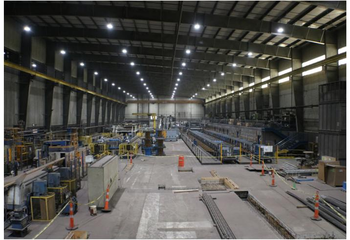
The LED installation was able to achieve a 20 foot-candle increase, resulting in a safer work space.
